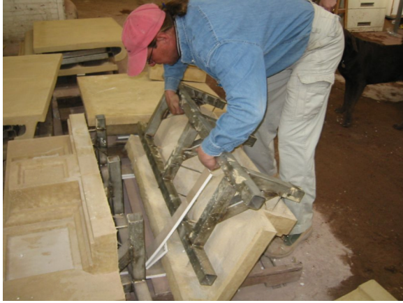
Figure 19. Stainless steel subframe on back of a cornice unit.
