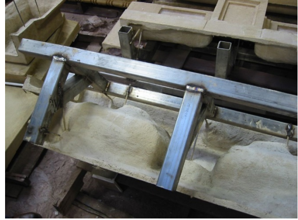
Figure 20. Close up of stainless steel subframe.
