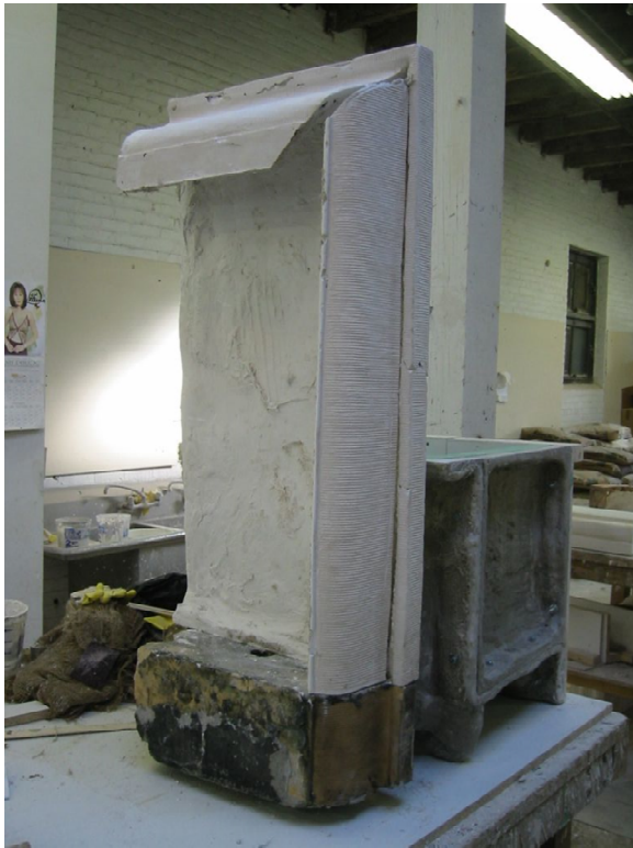
Figure 14. Early replacement sample showing alignment with original terra cotta.
