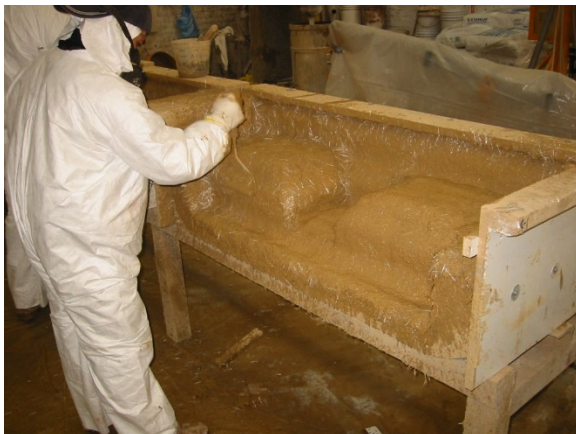
Figure 17. Back rolling fiber consolidation
