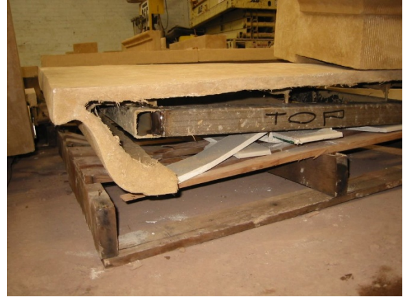
Figure 24. Side view of top course with stainless steel support frame.
