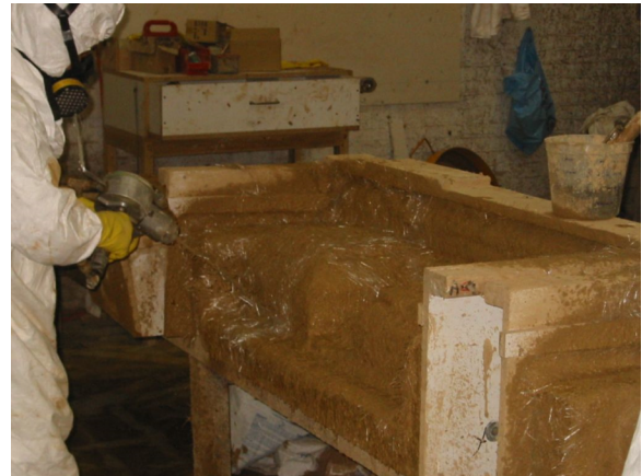
Figure 16. Note visible glass fibers in the mix
