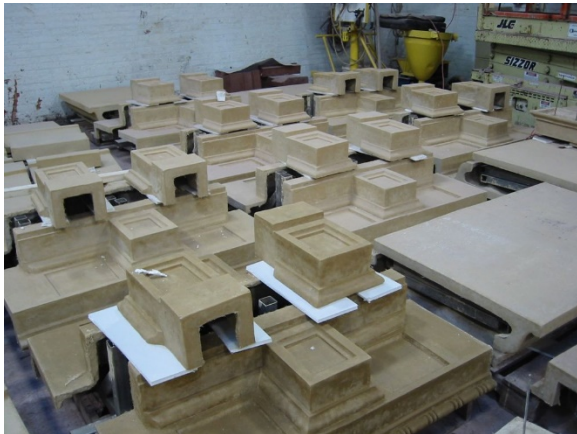
Figure 21. Curing and storage of the GFRG. Note the variety of shades indicating relative rate of drying
